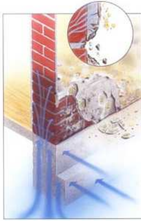
Fig. 2. Rising moisture created from the direct connection between soil and masonry.
