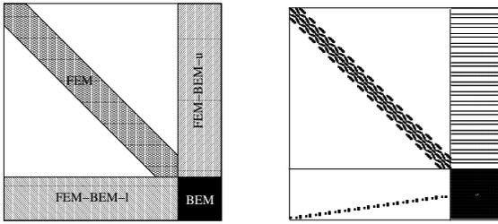
Fig. 3. The FEM-BEM matrix structure
