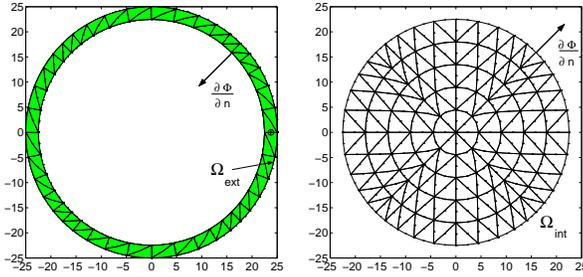
Fig. 2. Interface between two FE sub-regions
