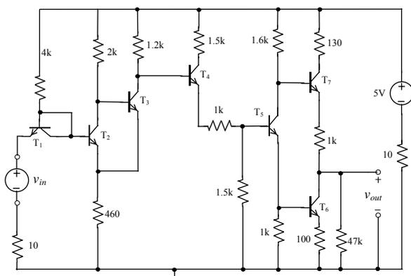
Fig. 2. The Schmitt trigger.
