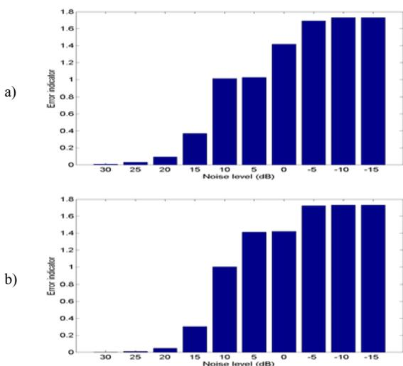
Fig. 5 The dependence of error of whitening on the SNR value for different signal compositions: a) 3 sinusoidal and 7 noise signals, b) 3 sinusoidal and 97 noise signals,
