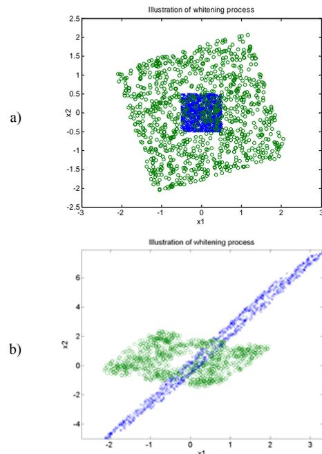
Fig.1 Scatter plots illustrating the whitening transformation for two sensor signals
