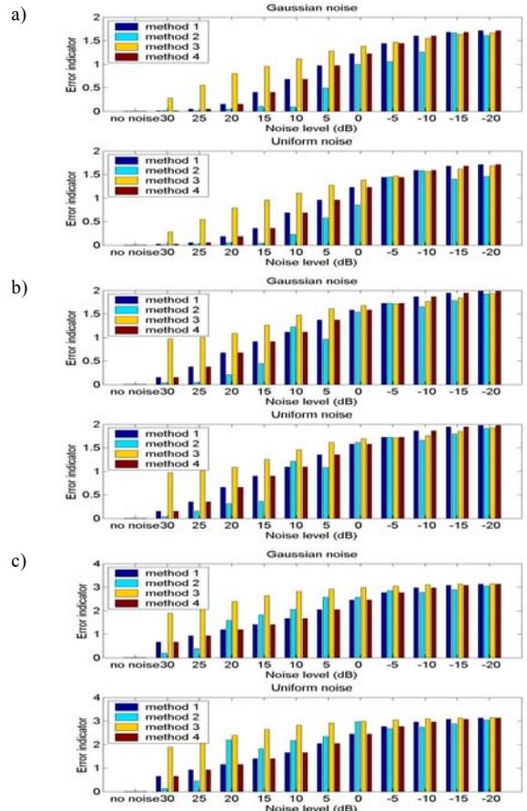
Fig. 4 The dependence of whitening error indicator on SNR for different noise distributions and different signals: a) 3 sinusoidal signals, b) 4 independent speech signals, c) 10 dependent speech signals all corrupted by noise (in all cases dimension of signal plus noise was equal 10)
