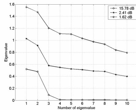
Fig. 2 The distribution of the eigenvalues of the correlation matrix at three different SNR values for the set of signals containing 3 noisy signals and 7 random noise components
