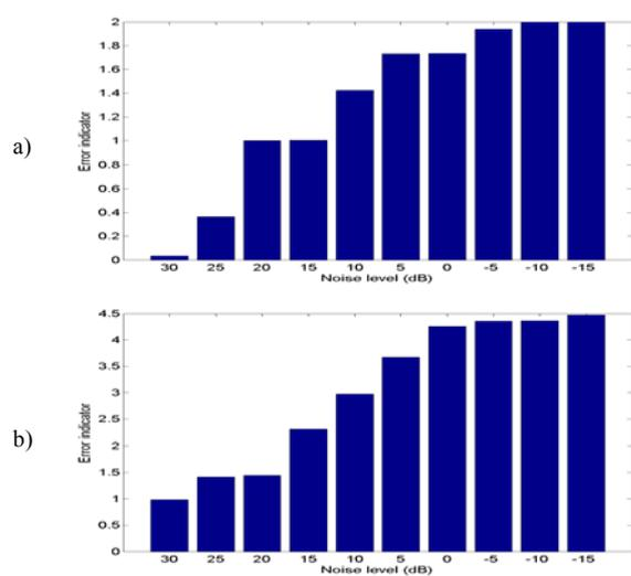
Fig. 6 The dependence of error of whitening on the SNR value for different type of signals: a) 4 independent speech and 96 noise signals, b) 20 dependent speech and 80 noise signals
