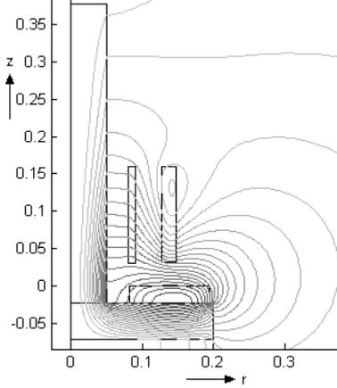
Fig. 4. Distribution of electromagnetic field during the dosing regime (for the lowest level of zinc)
