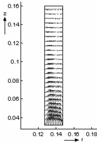
Fig. 5. Distribution of the Lorentz forces during the dosing regime (for the lowest level of zinc)
