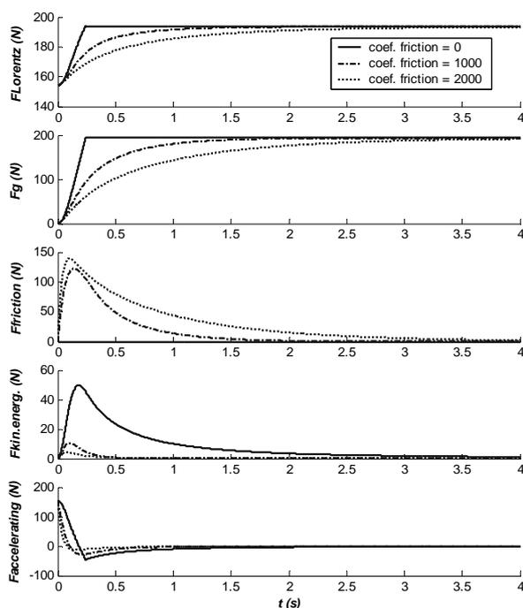
Fig. 9. The time dependence of forces occurring in (5) at the beginning of dosing for three different friction coefficients
