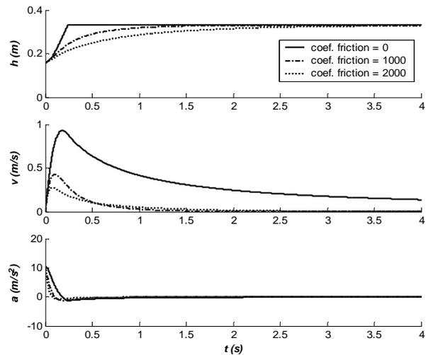
Fig. 8. Time evolution of height of the zinc level, velocity and acceleration at the beginning phase of dosing for three different friction coefficients
