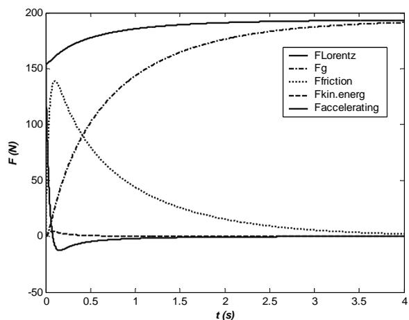
Fig. 10. The time dependence of forces occurring in (5) at the beginning of dosing for friction coefficients 2000.
