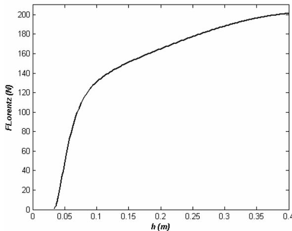
Fig. 6. Dependence of the total vertical Lorentz force in the zinc level
