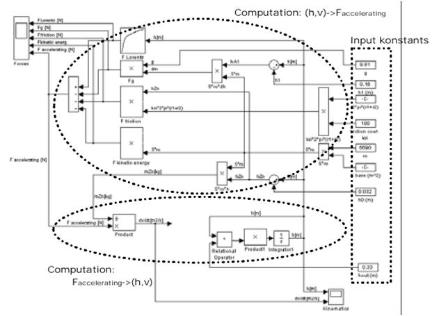
Fig. 7. Computational model built in SIMULINK.
