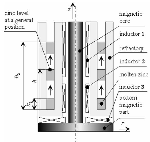
Fig. 2. A simplified (2D) arrangement of the feeder (without the inlet and outlet)
