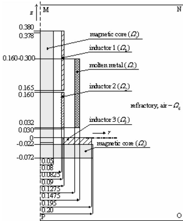
Fig. 3. Geometry of the zinc feeder
