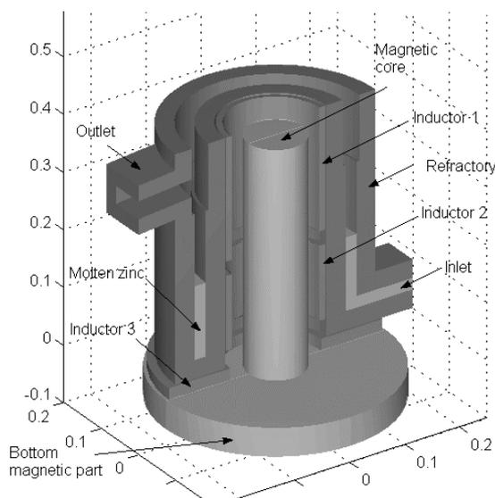
Fig. 1. Basic disposition of the electromagnetic feeder
