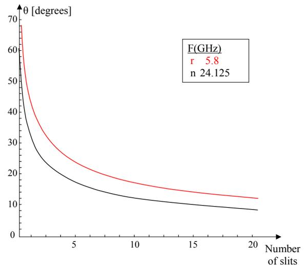
Figure 3. The slope  $\theta$ , depending on the number of slits, for a centered slit sloped on the large side of the wave-guide (for different frequencies).
