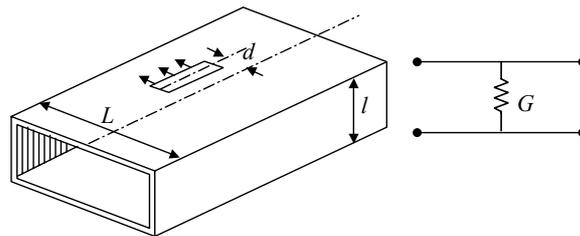
Figure 1. Longitudinal slit and its equivalent circuit.
