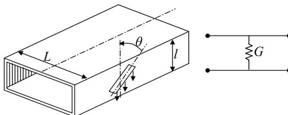
Figure 2. Sloped slit and its equivalent circuit
