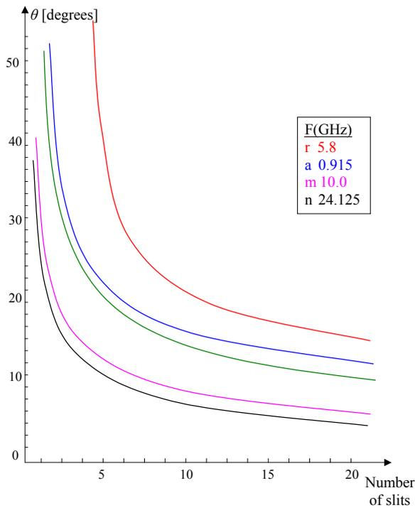
Figure 4. The slope  $\theta$ , depending on the number of slits, for a centered slit sloped on the small side of the wave-guide (for different frequencies).
